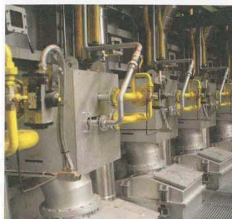
Cover photo: Tenova FlexyTech® TRGX burners at a reheating furnace
